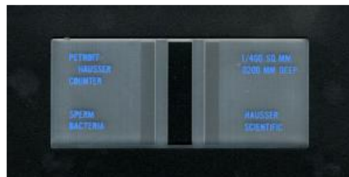
Fig.1. Petroff - Hausser counting chamber
